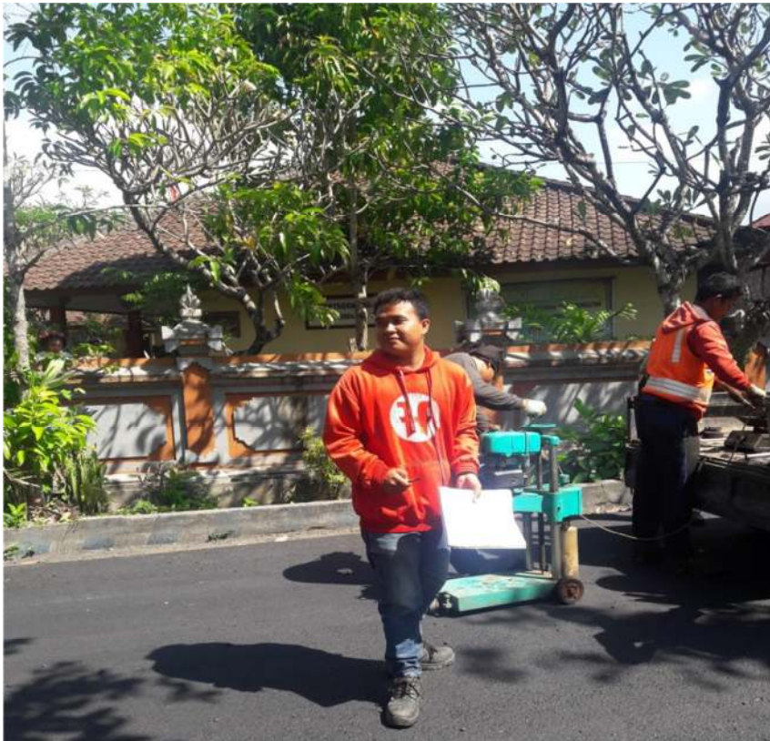
Lampiran F4: Pengambilan sampel hasil Core
